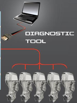
**Engine Monitoring** - for J1939 or NMEA2000 protocol for up to 5 engines.
